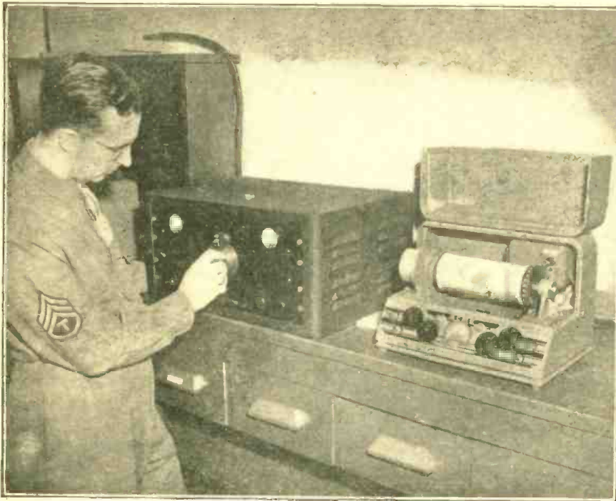
The facsimile apparatus with which picture news of American victory was rushed to the United States. The picture is formed on the cylinder at the right.
