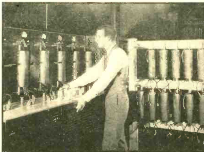
Phanotron tubes being tested in General Electric's Electronics Department before shipment to industrial war plants where they will be used for power rectification, to change A-C electric power to D-C, which is much more convenient for workers using small motors, such as are used on machine tools.
